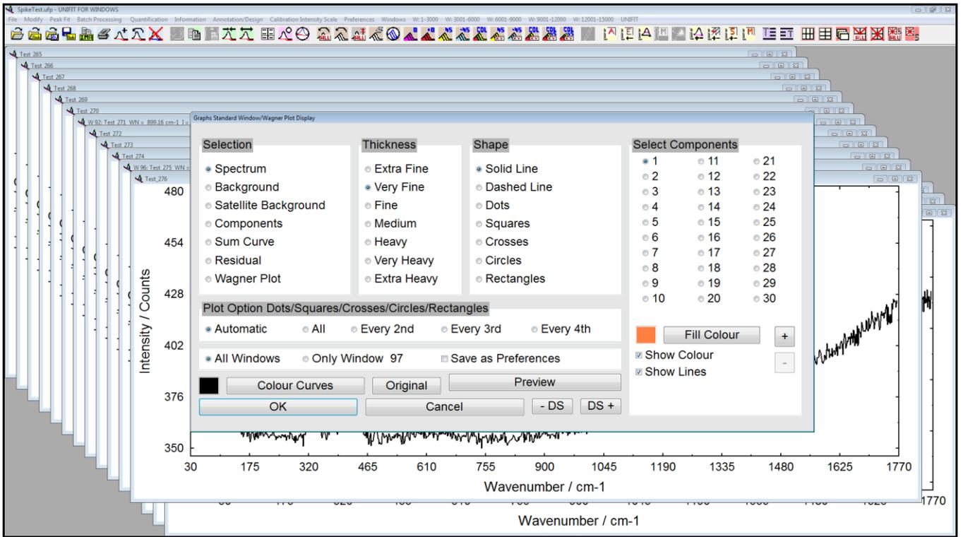
**Fig. 3.** Screen shot of the dialogue for the definition of the graphs of standard windows, the option 'Plot Option Dots/Squares/Crosses/Circles/Rectangles' is new
