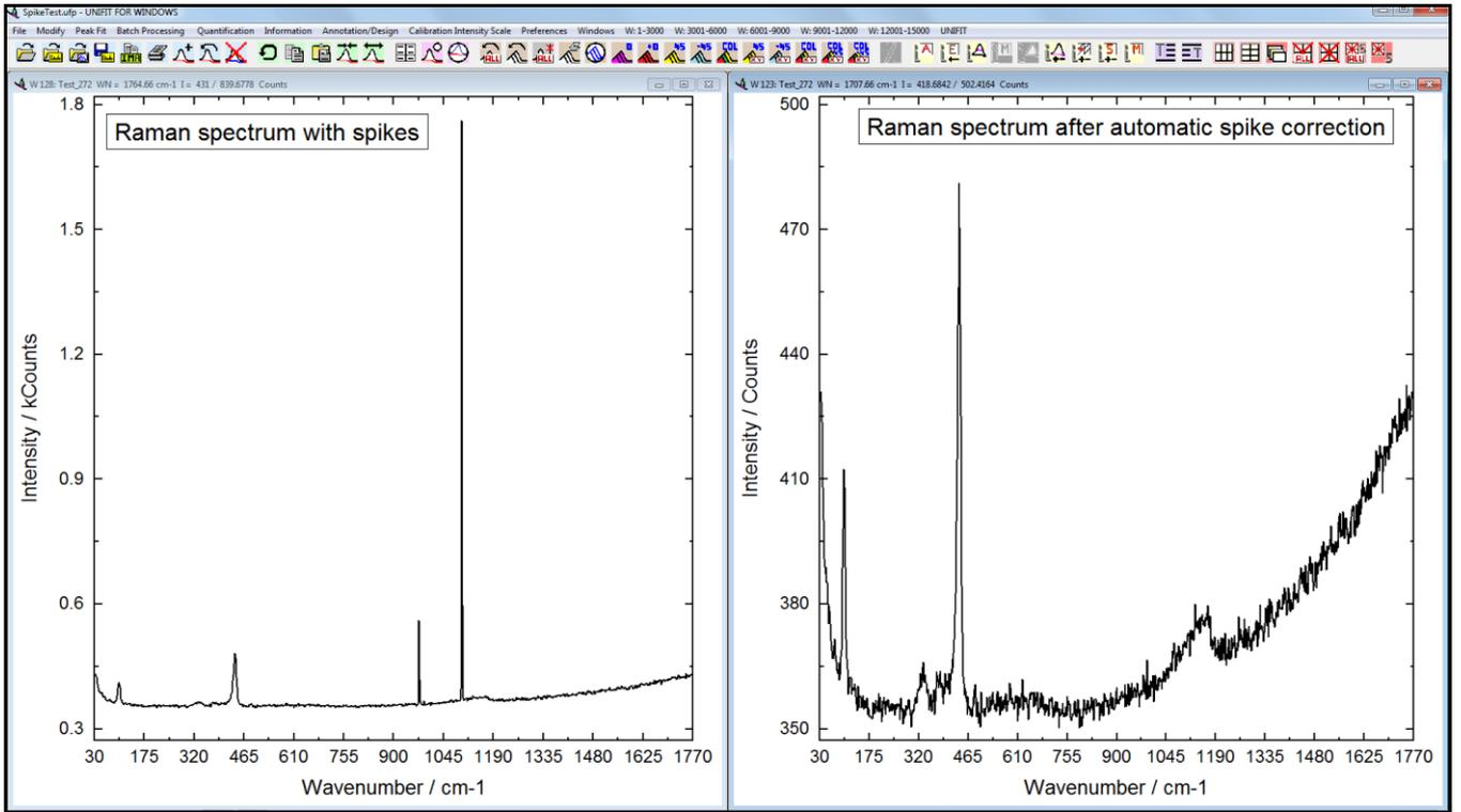
**Fig. 7.** Screen shot: Left: Raman spectrum with spikes (see also Fig. 6), right: Raman spectrum after the automatic spike correction
