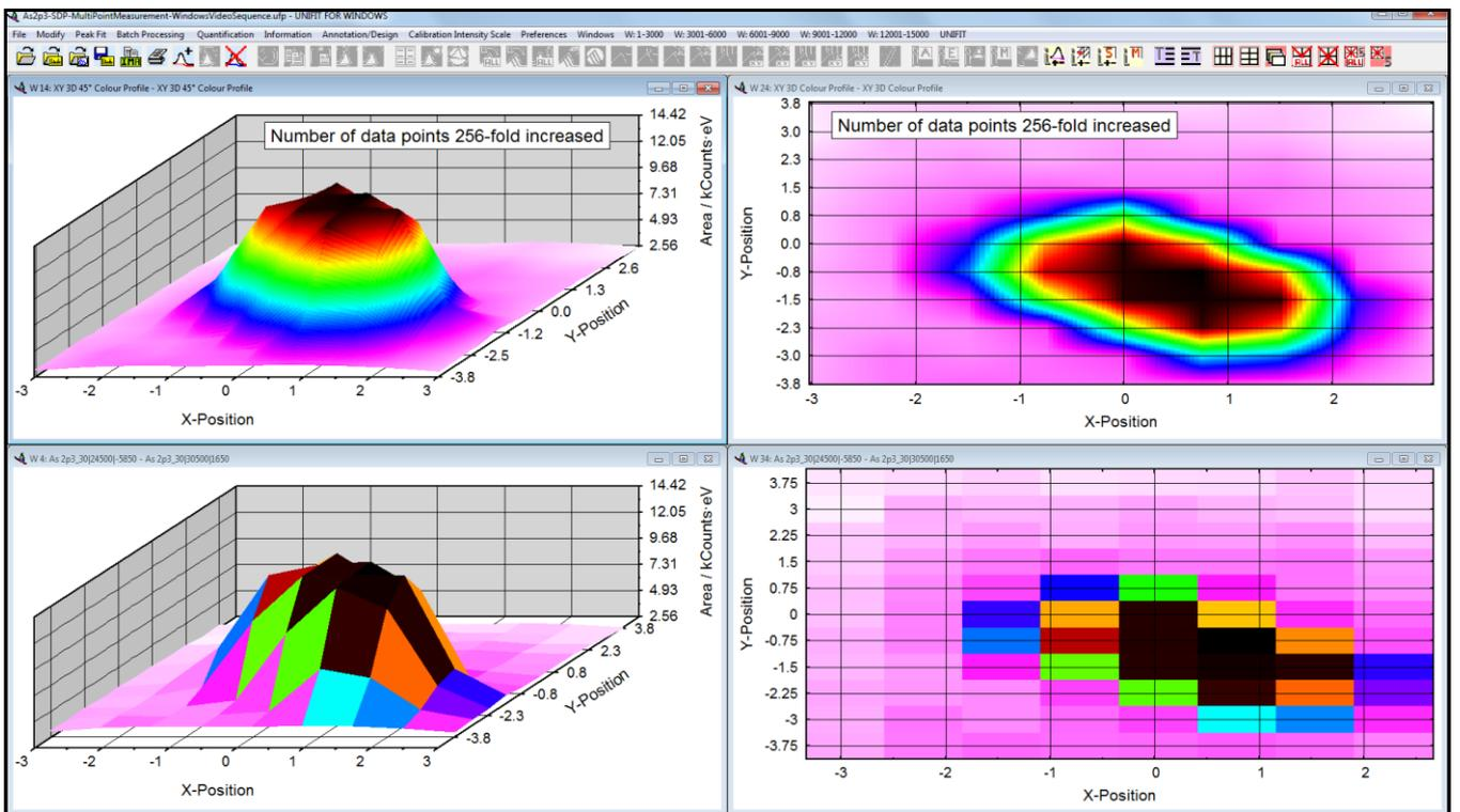
**Fig. 2** Screen shot of four 'XY 3D Colour Profiles': bottom left: 'XY 3D 45° 3D Colour Profile' without modification, top left: 'XY 3D 45° Colour Profile' after 256-fold increasing of data points, bottom right: 'XY 3D Colour Profile' without modification, top right: 'XY 3D Colour Profile' after 256-fold increasing of data points
