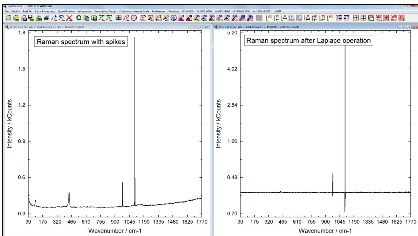
**Fig. 6.** Screen shot: Left: Raman spectrum with spikes, right: corresponding Raman spectrum after the improved Laplace operation, the sharp positive peaks show the position of the spikes
