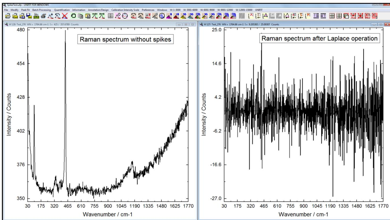
**Fig. 5.** Screen shot: Left: Raman spectrum without spikes, right: corresponding Raman spectrum after the improved Laplace operation
